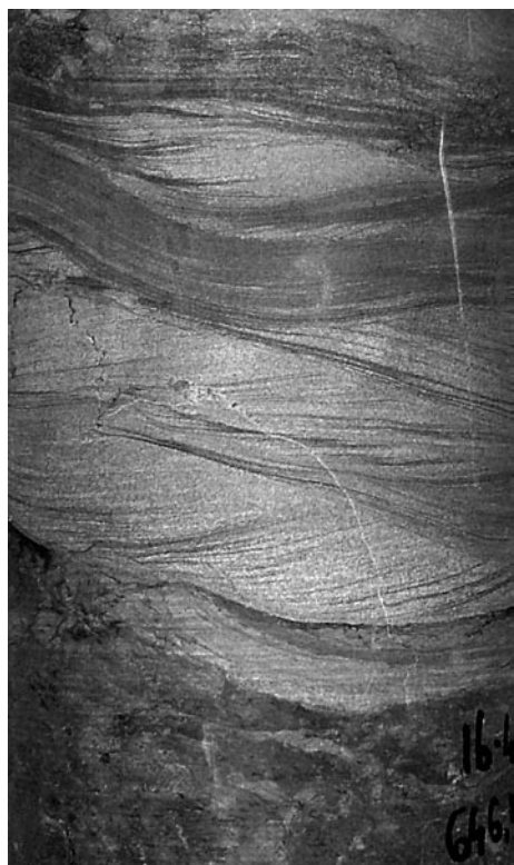
Fig. 11. Ripple cross-bedding in siltstone overlying claystone with a pedogenic structure. Surface of drilling core from borehole Ib-4, 646 m, image width 5 cm.
