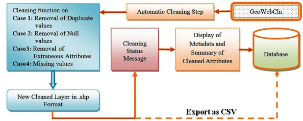
Fig. 3. Data cleaning process using GeoWebCln tool.
