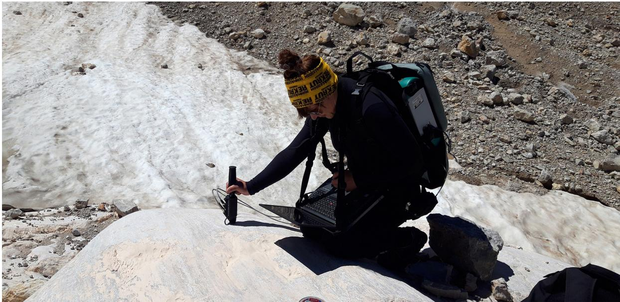
Fig. 3. The spectroradiometer ASD FieldSpec used in weathering studies in front of Hallstätter Glacier in the Alps (photo M. Dąbski).
