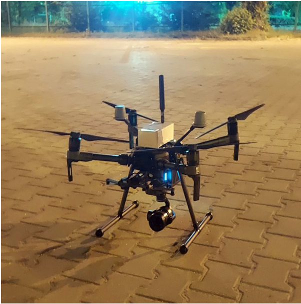
Fig. 1. DJI Matrice 210 RTK drone with its proprietary measuring device (photo D.Karpińska).
