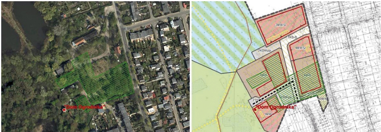
Fig. 5. Proposed landscape changes at Leszczyńska Street. On the left – the current land use in the vicinity of the gardeners' house ( dom ogrodnika ) and the former brickyard with the surrounding greeneries. Green colour indicates trees for cutting down. On the right – the draft of the zoning plan with areas intended for built-up (in red) and roads (in black).
