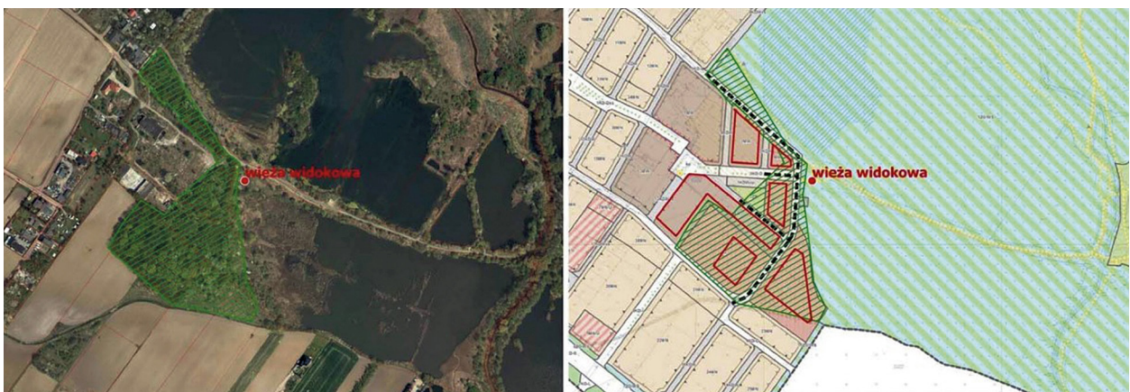
Fig. 4. Proposed landscape changes at Mieszyńska Street. On the left – the current land use in the vicinity of the lookout tower ( wieża widokowa ) and the former brickyard with the surrounding greeneries. Green colour indicates trees for cutting down. On the right – the draft of the zoning plan with areas intended for built-up (in red) and roads (in black).
