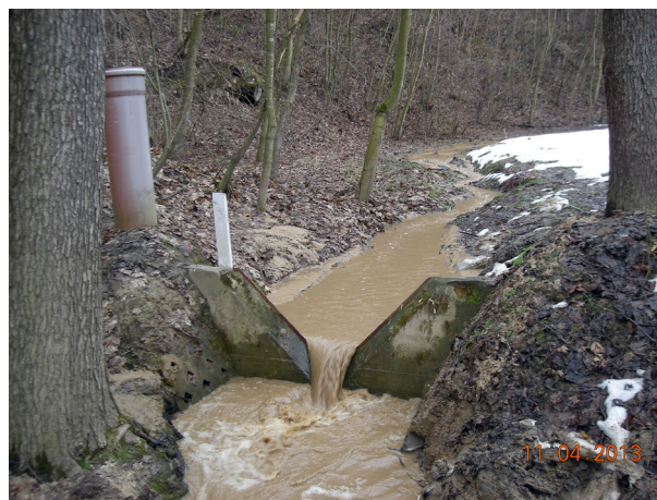
Fig. 2. Measurement of snowmelt flow at the hydrometric cross-section closing the gully catchment (photo by J. Rodzik).
