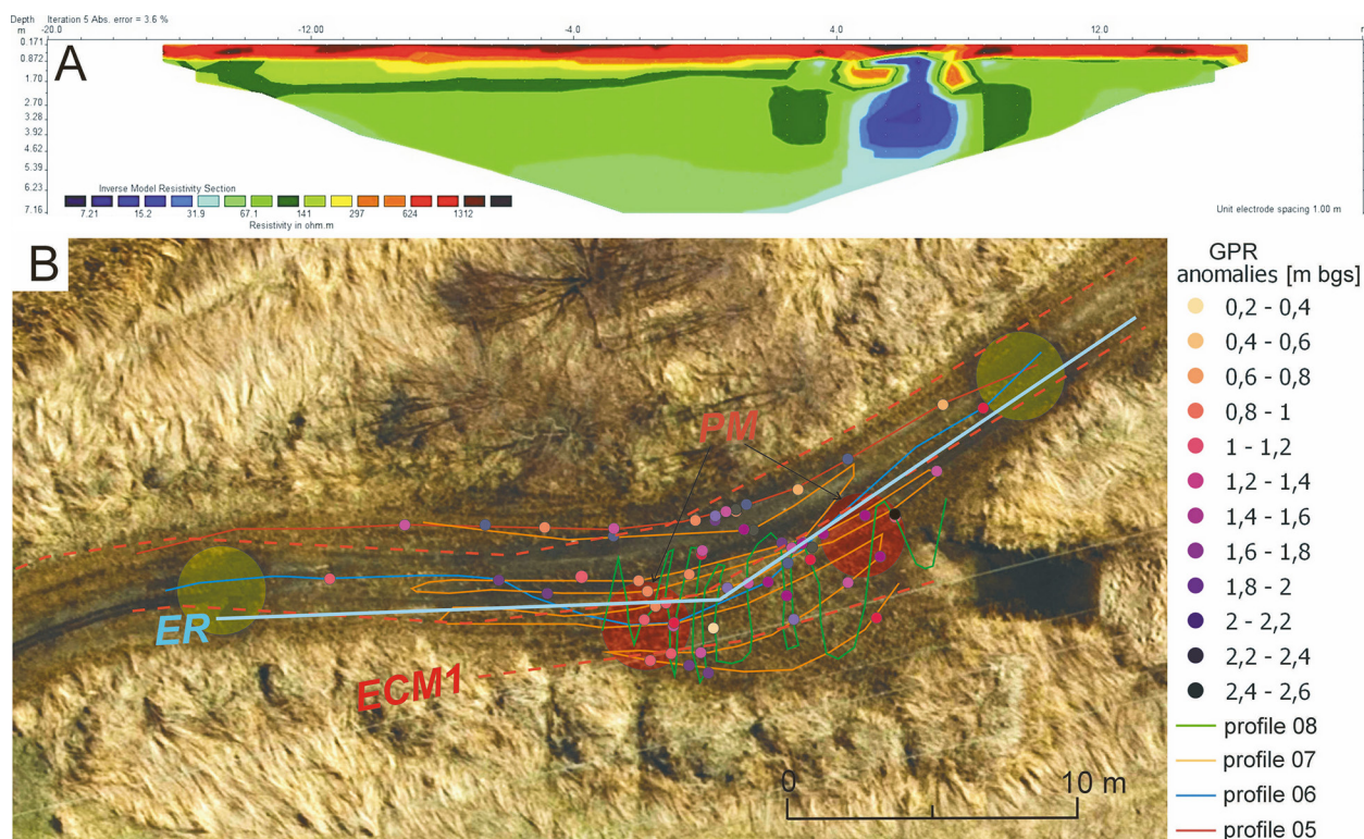
Fig. 11. Experimental area 3: A – diagram presenting electrical resistivity tomography results obtained in a wetland; B – profiles lines ECM1, GPR, ER and two concentrations of PM signal occurrence (red circles). Large yellow circles – probable remnants of the UXB fall. The profile described as ECM1 is shown in Fig. 8B.
