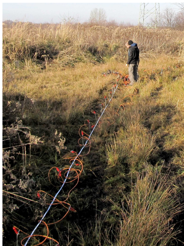
Fig. 5. Electrical resistivity tomography using ABEM's LUND Imaging System (photo: J.M. Waga).
