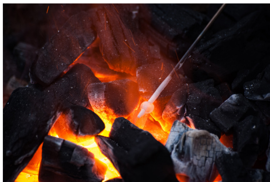
Fig. 4. The making of the base bead (phot. M. Rutkowski) A – Applying glass on mandrel, B and C – shaping the bead using gravity
