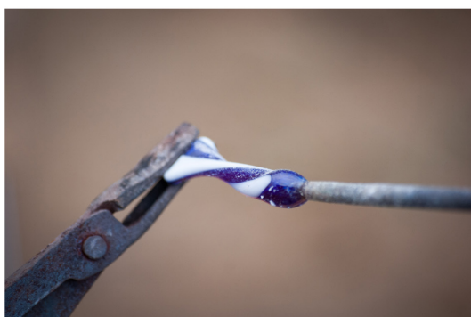
Fig. 9. The making of reticella (phot. M. Rutkowski) A – cylinder shaping, B – cutting and twisting
