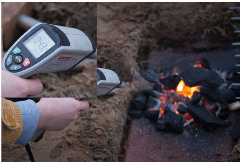
Fig. 3. The prepared hearth (phot. M. Rutkowski) A – Placing of bellows, B – value of temperature measurement
